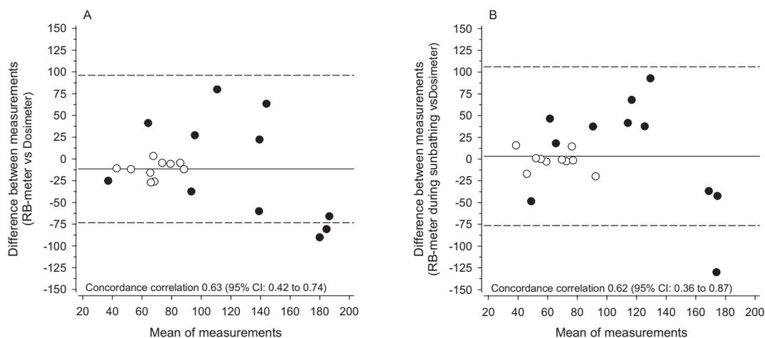
**Figure 1.** Bland–Altman plots for personal UV-B dose assessments using the RB meter combined with diary records *versus* dosimeter results (A) and using RB meter recordings during sunbathing hours *versus* dosimeter results (B). Dotted lines show 95% limits of agreement. Patients received heliotherapy either in January (empty circles) or in March (black circles).
