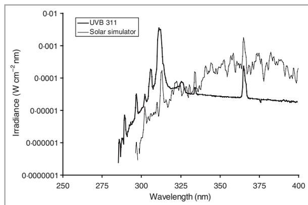
**Fig 1.** Spectral irradiances of the narrowband ultraviolet B (UVB) equipment (UVB 311; Waldmann UV 7001 cabin or 801KL panel with TL01 tubes; Waldmann) and solar simulator (Philips) used in the study. The optimal wavelength for vitamin D synthesis in the skin is 297 nm.
